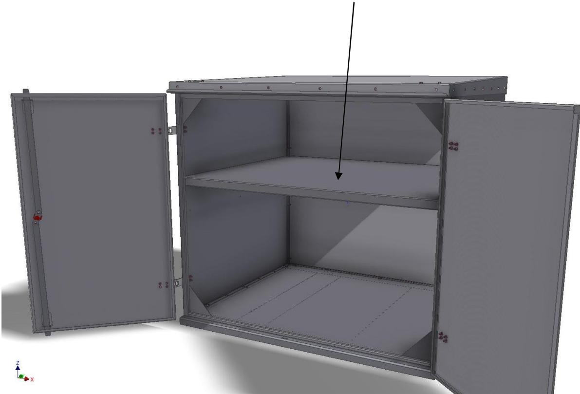
The second thing you need to do is mark the holes of the shelf on the side-panels and back-panel of the cargo box.
