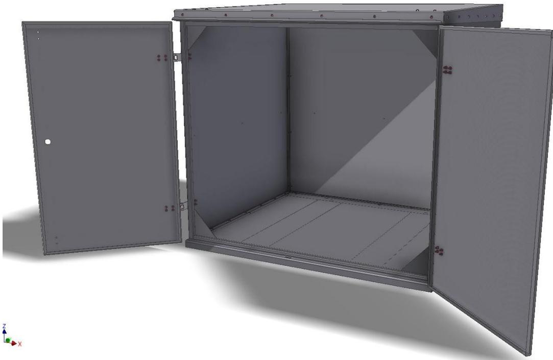
Mounting the hinge from outside. Use the M6\*12 bolts, nuts and washers
