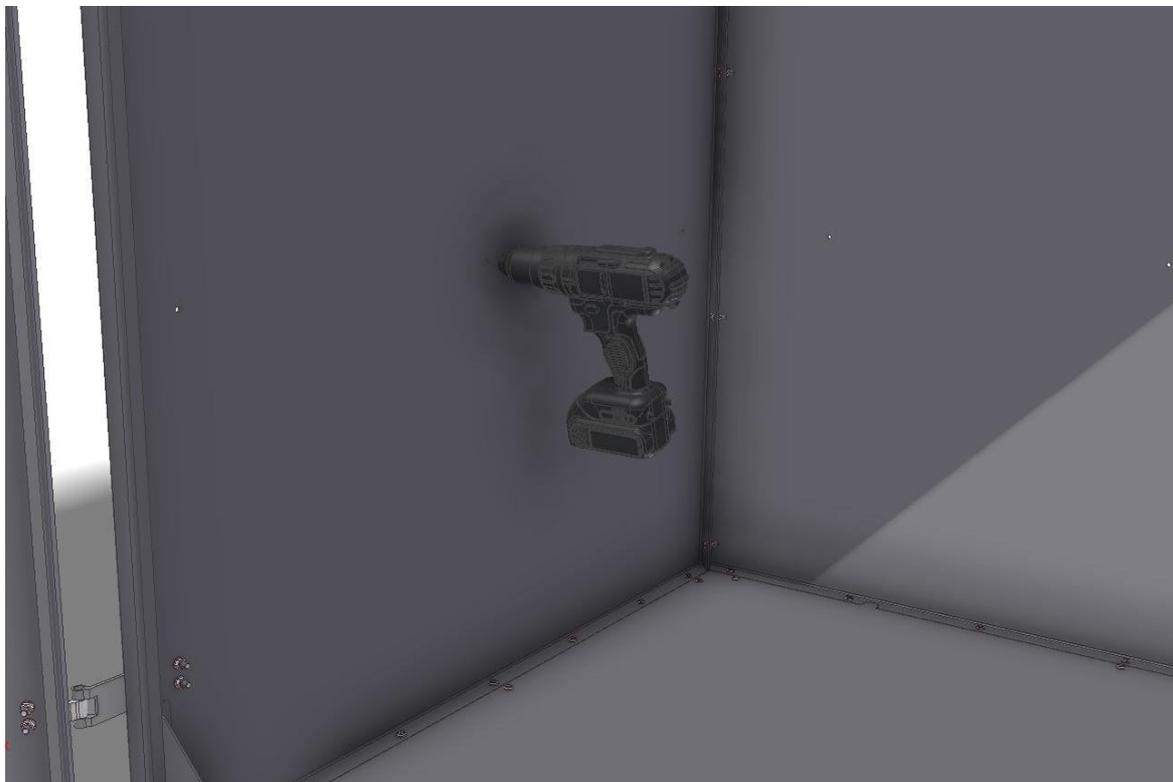
Now you can bolt the shelf into the Cargo-box using bolts, nuts and rivets. Use the M6\*12 bolts, nuts and washers
