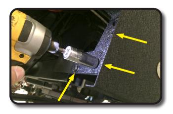
Before tightening the bumper, you can adjust the bumper to your specifications by using the slotted holes in the bumper and bracket. Once bumper is adjusted to your preferred location you may tighten all hardware.
