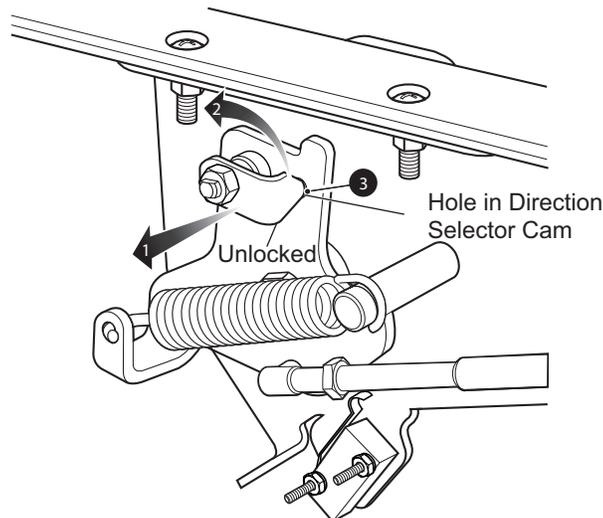
When in this position, the direction selector remains locked in the neutral position. To unlock the direction selector, pull the neutral lock pin handle out and rotate until the pointed portion of the handle fits into the hole in the direction selector cam.
