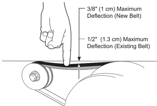
A **new** belt may be checked manually. A maximum deflection of 3/8" (10 mm) is acceptable. Tighten an **existing** belt to 75 - 80 lbs. (34 - 36 kg) tension using the same technique and inspect for cracking or wear. A maximum deflection of 1/2" (13 mm) is acceptable.
