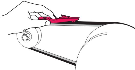
Tighten a **new** starter/generator belt to 115 - 125 lbs. (52-57 kg) tension when a gauge is applied half way between the two pulleys.
