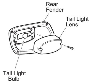
To replace the tail and brake light bulb, roll the rubber bezel from around the edge of the taillight and remove lens. Install replacement bulb and replace lens. To replace the tail and brake light bulb, remove hardware securing lens and remove lens. Install replacement bulb.
