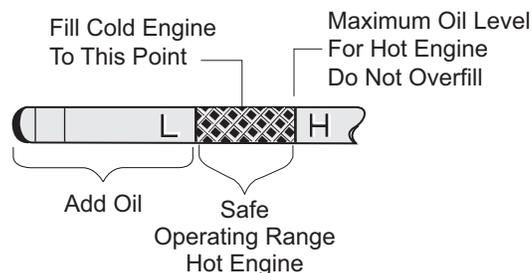
**Fig. 34 Check Oil Level on Dipstick**
