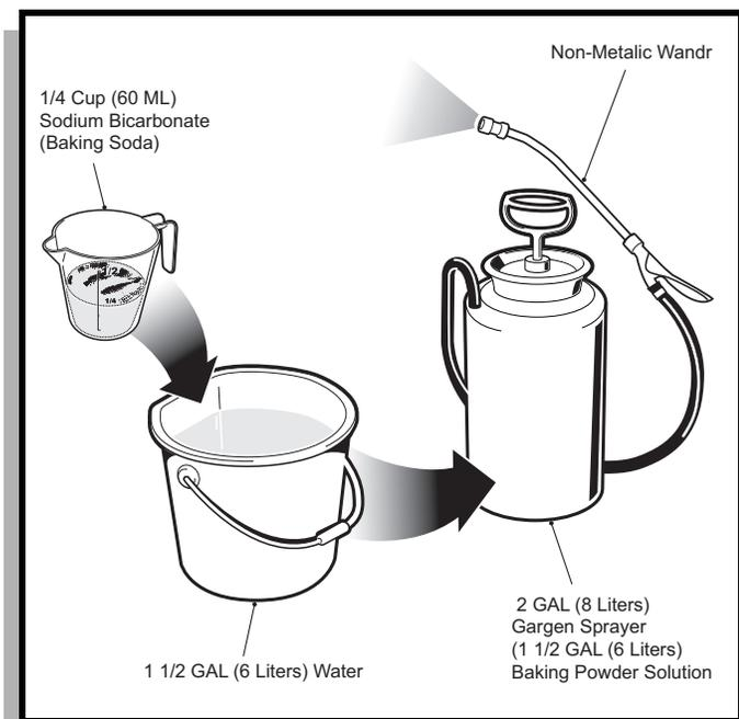
**Fig. 44 Preparing Acid Neutralizing Solution**
