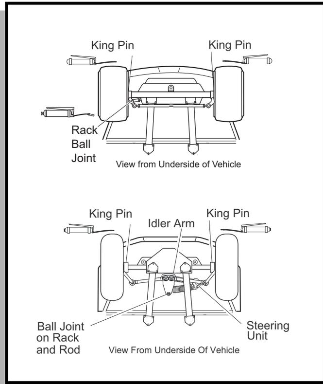
**Fig. 49 Lubrication Points**
