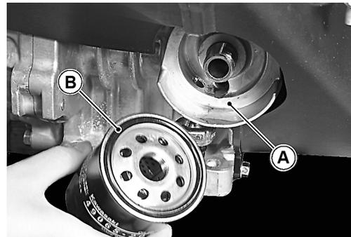
Fig. 38 Inspect Oil Filter
