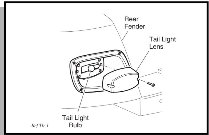
**Fig. 29 Tail and Brake Light Bulb Replacement**
