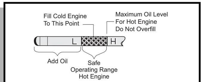
Fig. 21 Check Oil Level on Dipstick
