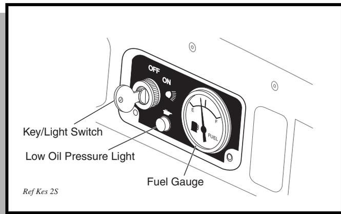
Fig. 2 Key/Light Switch and Fuel Gauge
