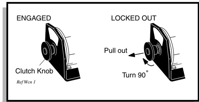
**Fig. 9 Winch Clutch Knob**
