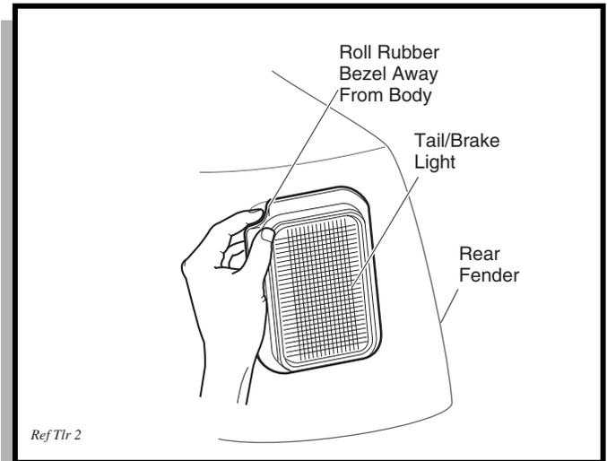
**Fig. 28 Tail and Brake Light Bulb Replacement**
