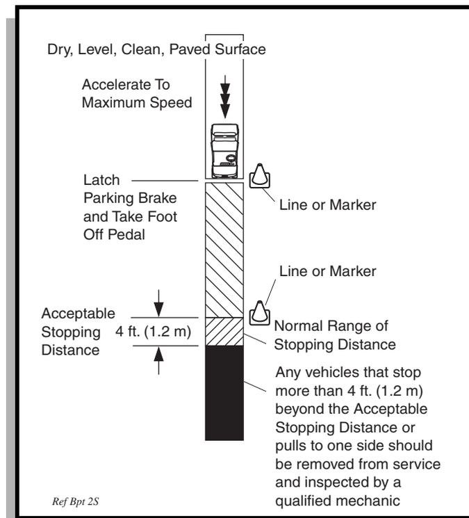
**Fig. 45 Typical Brake Performance Test**
