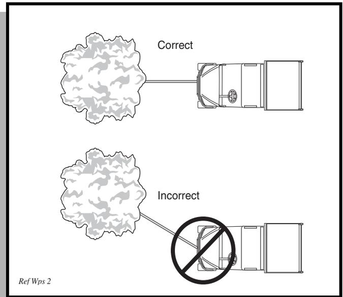
**Fig. 13 Do Not Pull at Angle**
