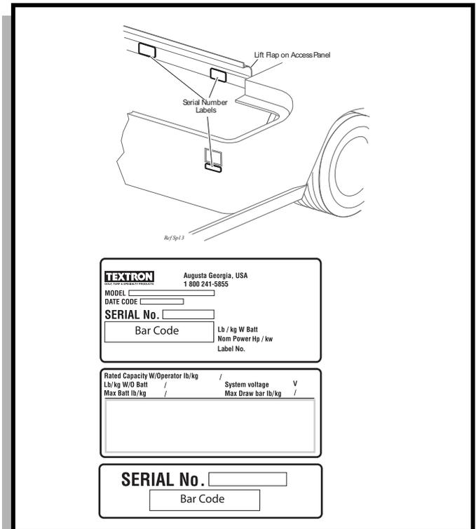
Fig. 31 Serial Number Label Location
