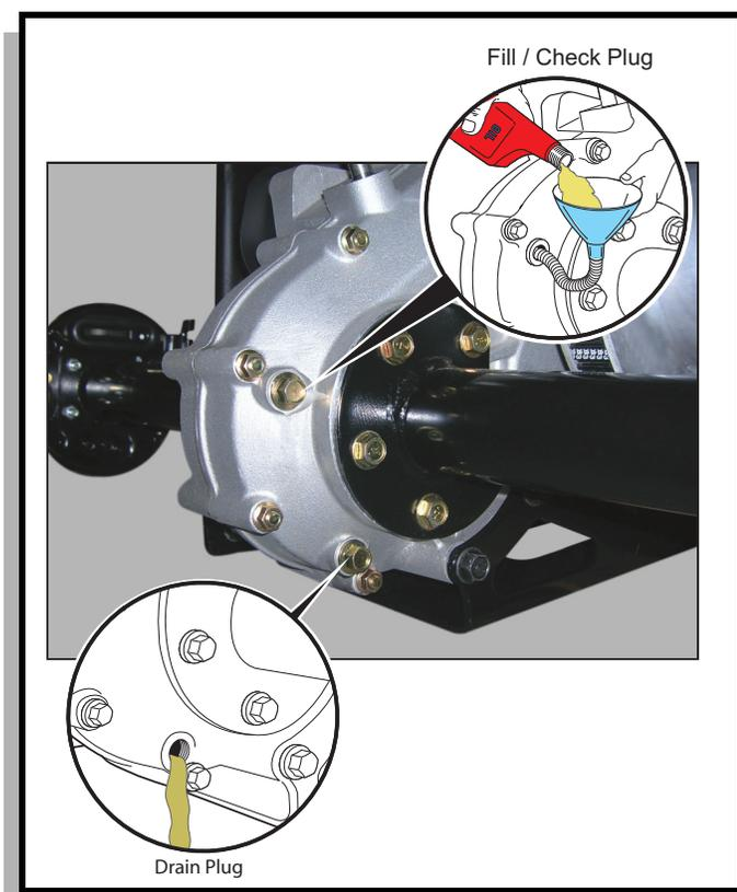
**Fig. 47 Add, Check and Drain Rear Axle Lubricant**
