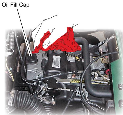
Fig. 36 Cleaning Top of Engine
