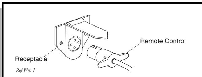
**Fig. 8 Winch Remote Control**
