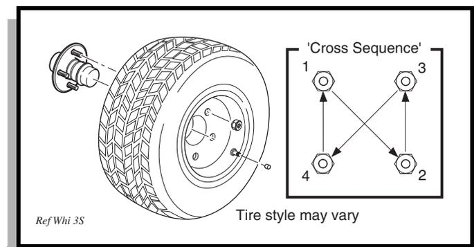
Fig. 25 Wheel Installation
