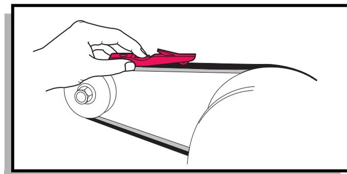
**Fig. 41 Check Belt Tension with Gauge**
