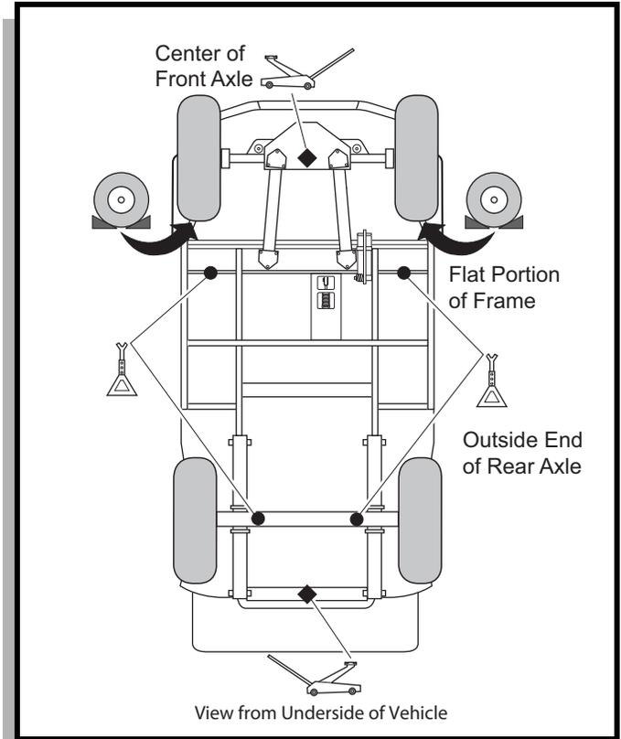
Fig. 24 Lifting the Vehicle
