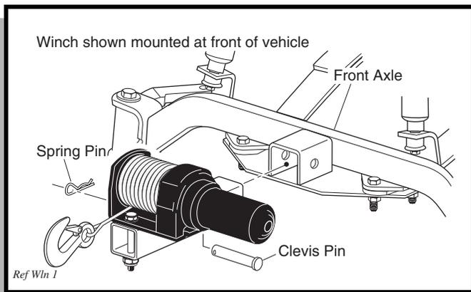
**Fig. 7 Winch Mounted to Vehicle**
